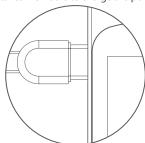
Please use the specific USB Type-C cable with the certified DC5V---1A adaptor to charge.
