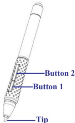
After using for a period of time, the refill will wear out. At this time, you can replace a new one that is included in the packaging box. The replacement method is as follows:
